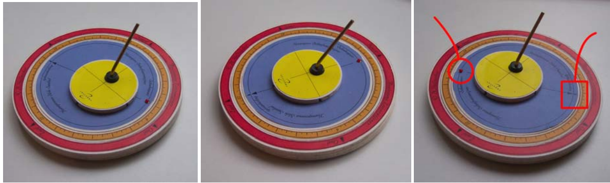
Figure 8: The homogeneous analemmatic sundial with polar style. The style points to the north as usual. Left and middle picture: 2 positions of the central disc. Right picture: the shadow point (in the circle) and the arrow which marks the time (in the square).
